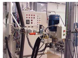
ADC's Meter, Mix, and Dispense machine: A two component machine with a dynamic mixhead
